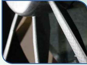
The QAD230 features a unique powerflow fan with "golf ball" dimpled blades which increases fan efficiency and air flow. At typical velocities of 1.7m/sec, the pressure drop
