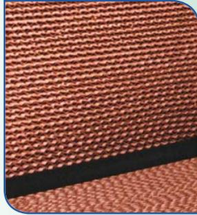
The QAD230 utilises a long-life, self supporting cellulose pad, impregnated with anti-rot salts, rigidifying saturates and wetting agents, with unique alternating, transverse flutes at different angles. The design creates highly turbulent mixing between cooling water and air, enhancing evaporative
